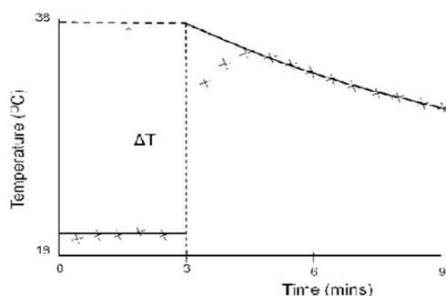
These graphs are constructed to eliminate the error that is due to heat loss to the surroundings. This gets a **more precise temperature change** from the cooling curve (for an exothermic reaction). The horizontal reflection in of the diagram on the left is the heating curve that occurs in an endothermic reaction. The same principle applies.
